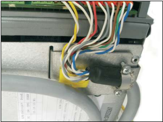
Figure 7.2.4: Connection of shielding (recommended)
